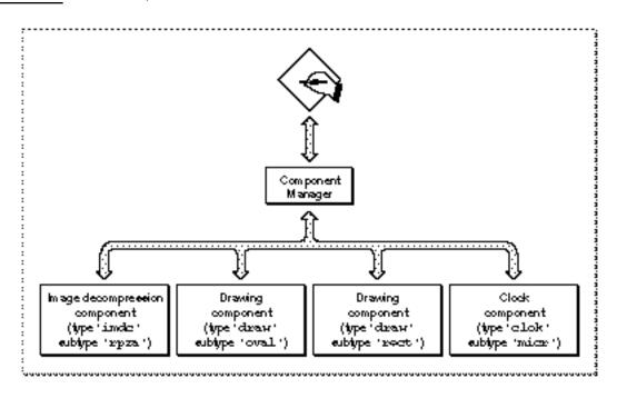
The Component Manager allows a single component to serve multiple client applications at the same time. Each client application has a unique access path to the
